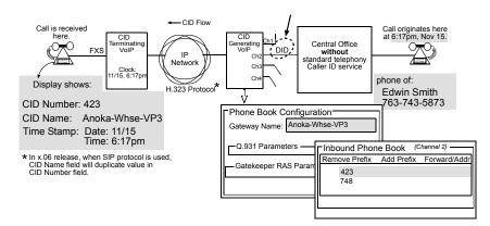
Figure 5: Voip Caller ID Case #5 – Call through telco central office without standard CID enters DID channel in H.323 voip system
